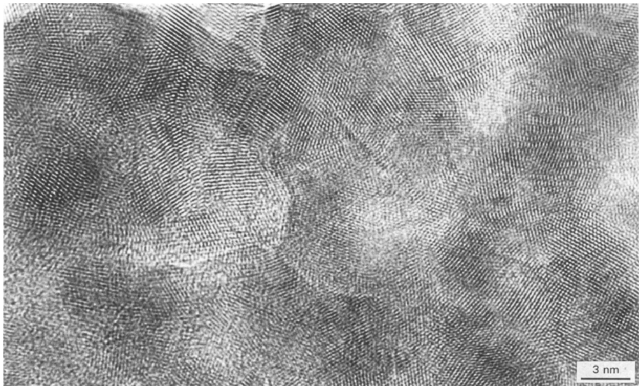
Figure 7 Nanocrystals formed after 60 h MA.
